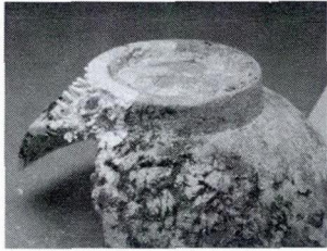
Fig. 1 Calcareous incrustation on the surface of porcelain
